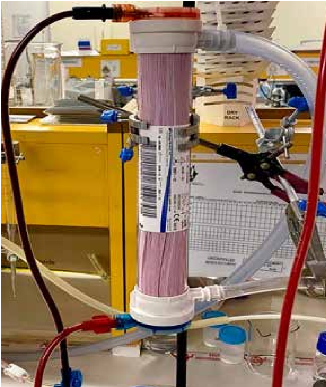
A hollow-fibre membrane dialysis cartridge is shown with dark deoxygenated blood entering the device at the top and bright red oxygenated blood exiting from the bottom of the device.
