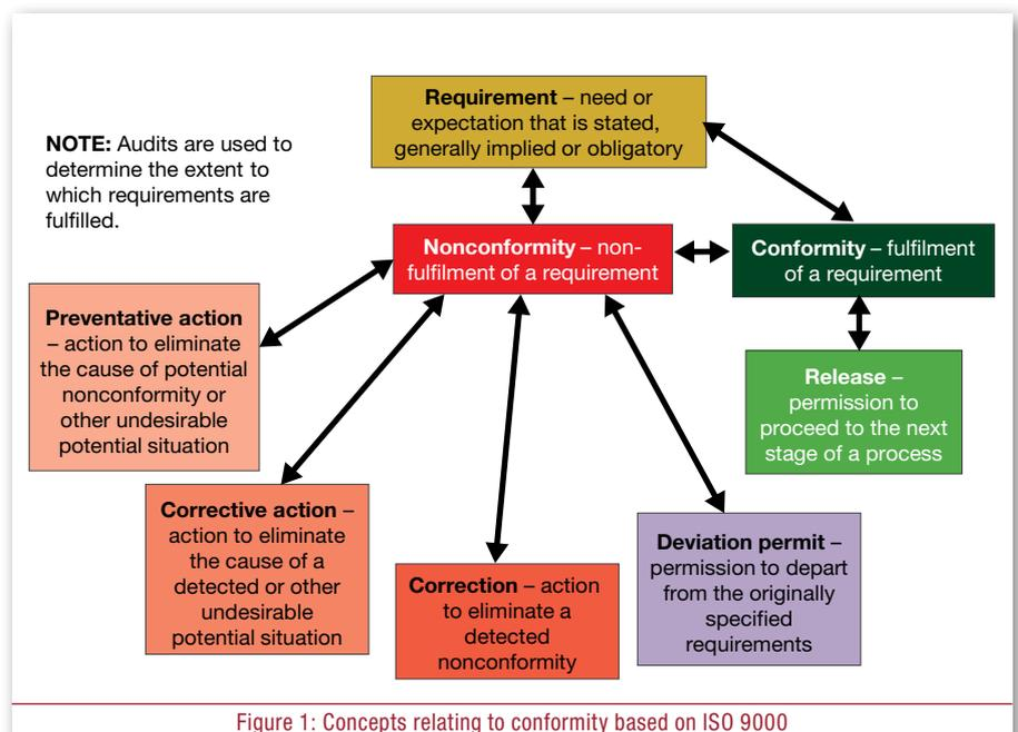
Figure 1: Concepts relating to conformity based on ISO 9000
