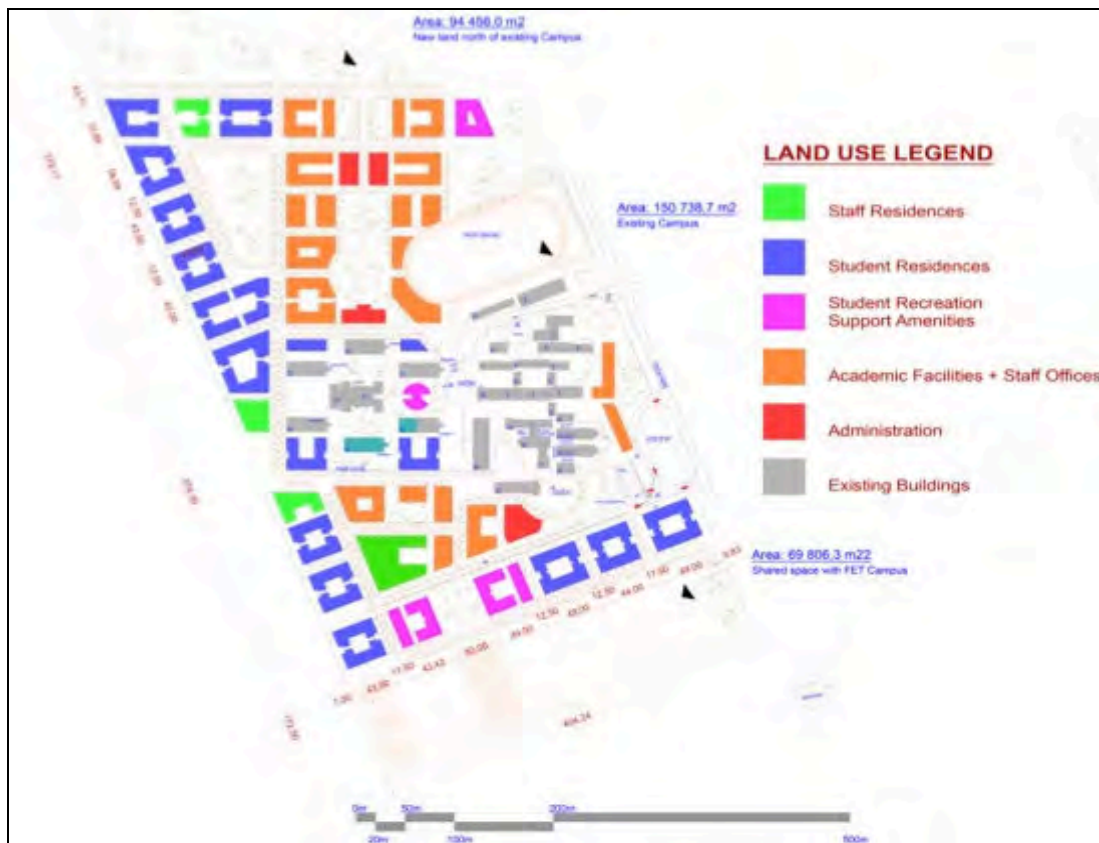
Fig 6.17: Spatial Design and Development Framework for the Siyabuswa Campus of the University of Mpumalanga. It shows the expansion of the expansion north and south to enable an expansion to approximately 3000 students.
