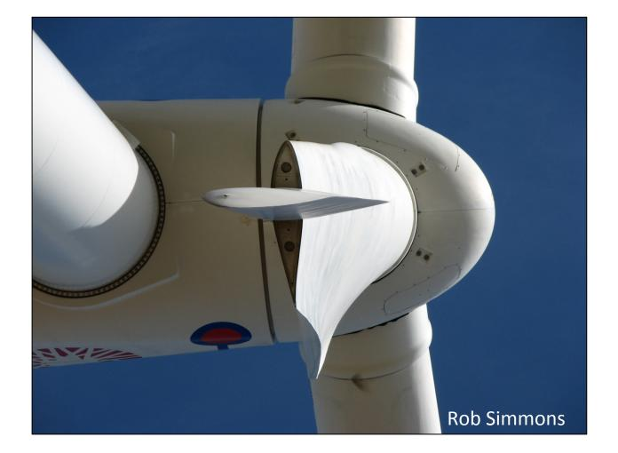
End-on-view of the turbine blade and "paddle" that acts as an air brake to stop the turbine rotating when winds become too strong.
