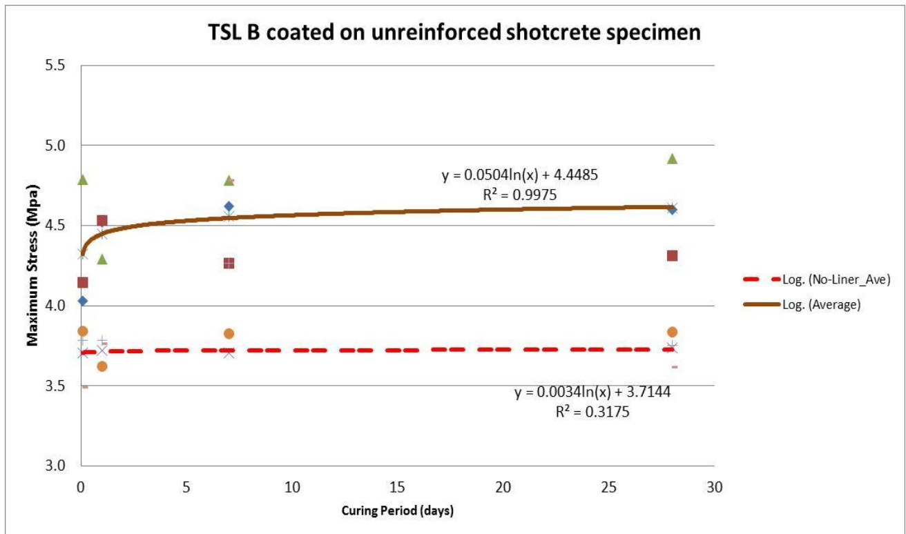
Figure D.3 Brazilian test on TSL B coated on unreinforced shotcrete specimen
