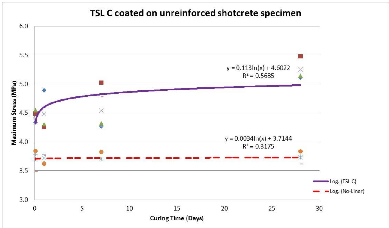
Figure D.5 Brazilian Test on TSL C coated on unreinforced shotcrete specimen
