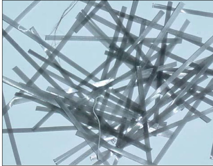
Figure 3. Polypropylene fibre used in the mix
