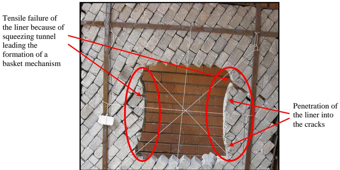
Figure 4.11 Tunnel squeezing before sidewall collapse
