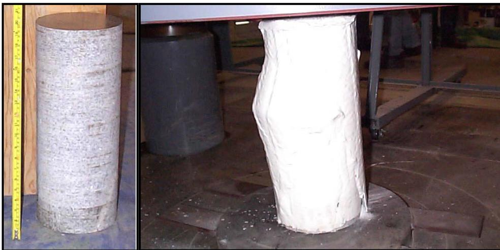
Figure 3. 3 Core sample and controlled lined rock core failure (Tarr *et al* 2006)
