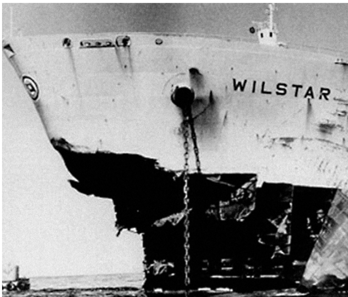
Figure 11: The ship Wilstar after an encounter with an extreme wave in the Agulhas current.
